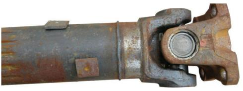
Rockford Driveline parts below you are able to cut the Original assembly apart 1/8" below the friction weld and replace the Weld Yoke, Flange Yoke & U-Joint with a servicable 1310 system.
